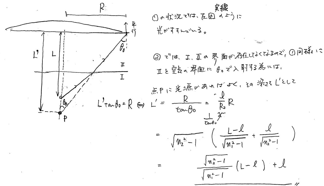
$$R_2 \text{ は } \frac{\sin \theta_0}{\sin \theta_\alpha} = \frac{R_2}{\sqrt{l^2 + R_2^2}} \Leftrightarrow \frac{1}{n_2^2} = \frac{R_2^2}{l^2 + R_2^2} \Leftrightarrow R_2^2 = \frac{l^2}{n_2^2 - 1} \Leftrightarrow R_2 = \frac{l}{\sqrt{n_2^2 - 1}}$$
